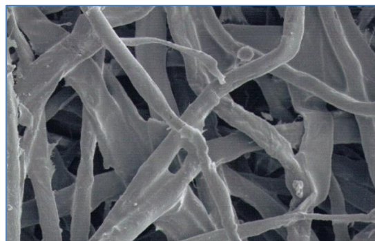
Unused paper element at x270 magnification
