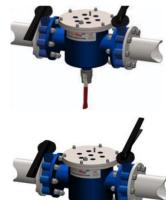
4. Either place a bucket underneath or connect a hose to the 1 ¼" drain valve on the underside of the unit. Remove the drain plug and open the drain valve.
