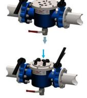
7. Replace the magnetic core and hand tighten the black tricone to retain.
