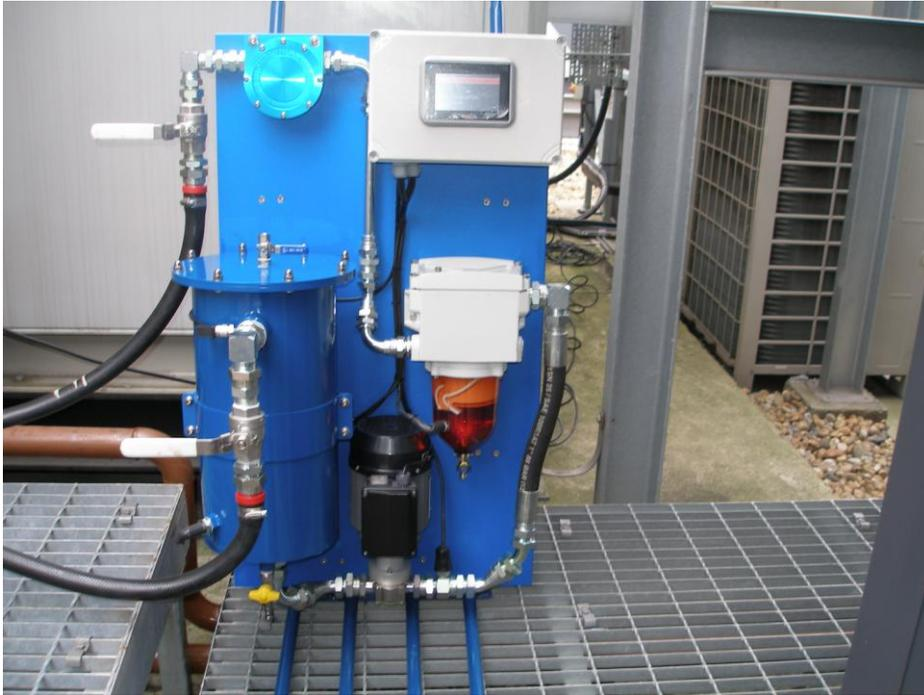
This site required me to manoeuvre the unit from ground level via a lift, then across a roof, over gravel and then up and over some gantries. The tank being polished is a standby generator day tank of 800ltrs, the fuel was visually dirty and laboratory results showed dirt/debris floating within the fuel. On completion of two hours running the polishing rig the fuel tested clean and dry. I was able to clean the fuel without taking the generator off line.
